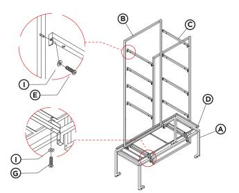
3 Place the remaining shelves (a) on top of metal rails (c). If necessary, slightly loosen bolts for the surrounding rails (c) to make placing shelves (d) easier. Fasten shelves from below using the medium length bolts (F).
