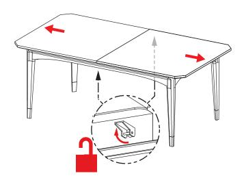
Lower the Table Leaf © on to the table. Making sure the dowels and holes align, push the table top ends back together against the table leaf. Finally, return the locks to the down position as shown.
